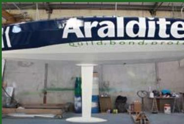
*The ‘Araldite’ Mini Transat racing boat is the smallest offshore racing boat allowed to cross the Atlantic and the first ever prototype to incorporate natural flax fiber in the composite structure*
