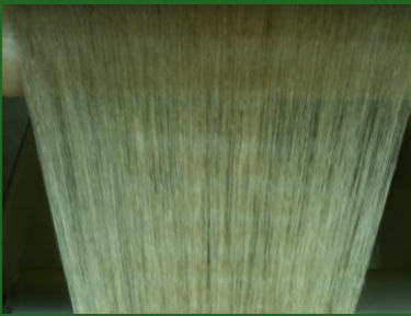
III FlaxTape on the production line
